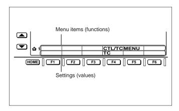
In the figure above, TC (time code) is selected as the setting for CTL/TC (time data selection), the menu item for button F4. This manual refers to this as "F4 (CTL/TC) in function menu HOME page is set to TC."
