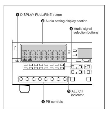
In the audio control section, you can select and display output signals for audio channels 1 to 8.
