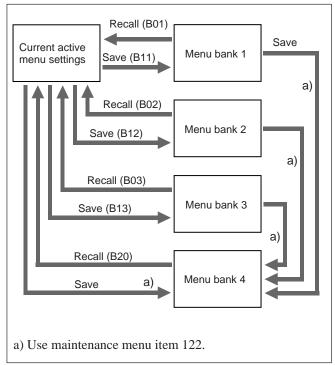
The current active setup menu settings as well as settings saved in menu banks are stored in separate storage areas for 525-line and 625-line modes.
