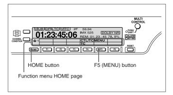
With the function menu HOME page showing in the menu display, press the F5 (MENU) button. The currently selected setup menu item is displayed in the menu display, with the menu item number flashing.
