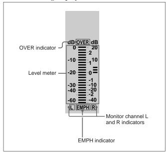
**OVER indicator:** While the unit is in playback mode, this lights when the level of the audio signal on the corresponding channel exceeds the maximum level that can be indicated on the level meter.
