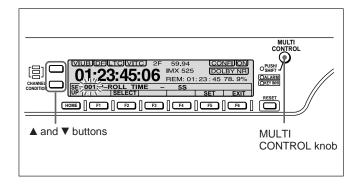
When the menu item number displayed in the menu display is flashing, you can change the menu item by turning the MULTI CONTROL knob.
