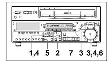
**1** Press the DMC/FEED button, turning it on.
